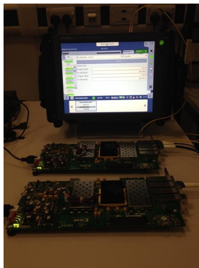
Figure 5-4: CPRI end-to-end test using two TSON edge nodes.
